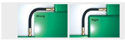
The same applies to hoses that are laid too close together. The hoses rub against one another. The wire braiding is no longer protected against corrosion and failure of the hose is only a question of time. Should it not be possible to rule out abrasion, it is possible to use hoses with highly abrasion-resistant outer covers.
