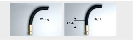
In some cases it is also possible to avoid exceeding the minimum bending radius by the use of suitable fittings.
