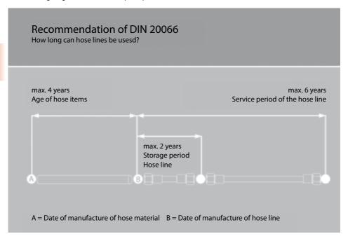
In practice, hydraulic hoses are stored according to the First In-First Out (FIFO) principle. FIFO defines a storage principle where the date of storage determines the date of retrieval from storage. This means that the hose that has been in storage longest is retrieved from storage first.
