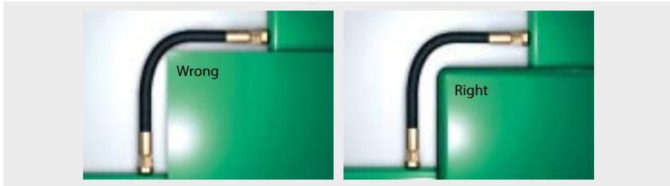
The same applies to hoses that are laid too close together. The hoses rub against one another. The braiding is no longer protected against external influences and failure of the hose is only a question of time. Should it not be possible to rule out abrasion, it is possible e.g. to use hoses with abrasion protection.
